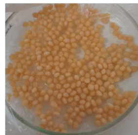
Figure 1. Photo of the synthesized Fe(III)-Alginate beads.
